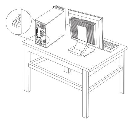
Figure 39. Installing a padlock
